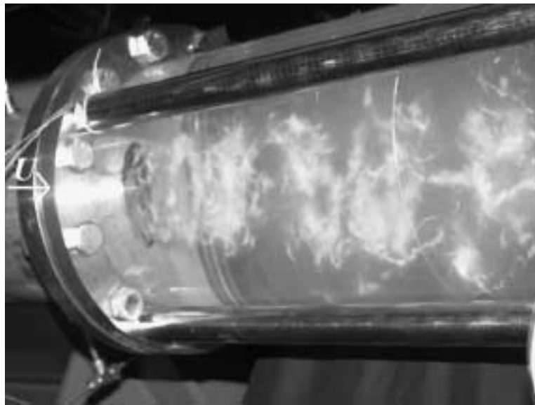
Fig. 15. From other experiments at EDF (Archer et al., 2002), visualization of a cavitating and whistling single-hole orifice ( d/D = 0.30 , t/d = 0.10 , D = 2.6 \times 10^{-1} \text{ m} ) with \sigma = 0.35 and U = 1.97 \text{ m s}^{-1} ( \Delta P = 5.3 \times 10^5 \text{ Pa} , P_1 = 7.2 \times 10^5 \text{ Pa} ).
