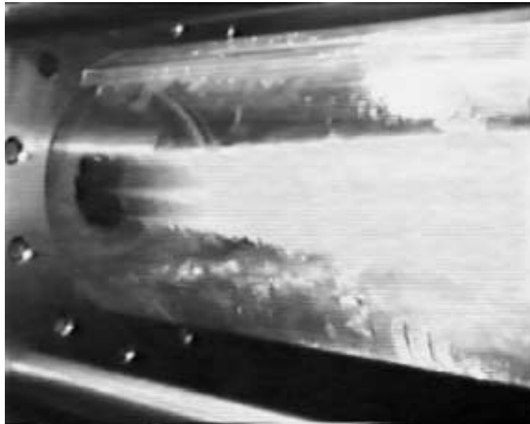
Fig. 16. From other experiments at EDF, visualization of the super cavitation regime for a single-hole orifice.
