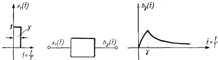
Fig. 5. Response of a system to an excitation in the form of a rectangular pulse
