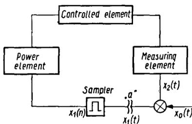
Fig. 23. Block diagram of a sampled-data control system
