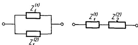
Fig. 2 Impedances  $Z_1$  and  $Z_2$  for the case in which the polynomials  $P$  and  $Q$  are of the second order
