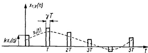
Fig. 3. Pulse signal generated by a sampler
