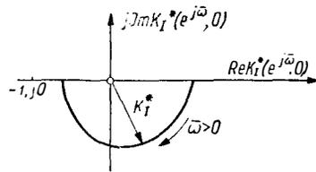
Fig. 22. Nyquist diagram of a simple sampled-data system
