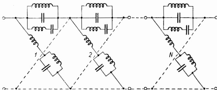
Fig. 11. Delaying long line
