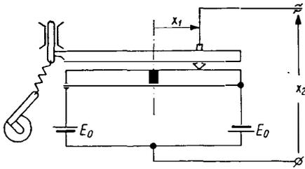
Fig. 13. Operation principle of the third-type sampler
