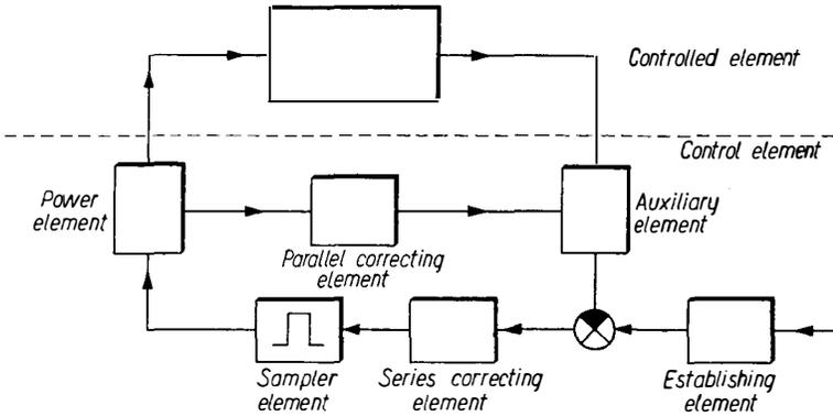
Fig. 1. Block diagram of a sampled-data control system
