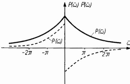
Fig. 13. Characteristic which ensures the monotonical function  $A^*(\bar{\omega})$
