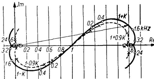
Fig. 8. Auxiliary functions necessary for graphical determination of the transfer function of a negistor
