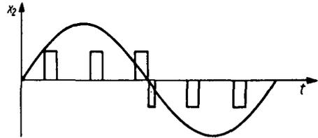
Fig. 14. Pulse signal in the case of a delay system with a key
