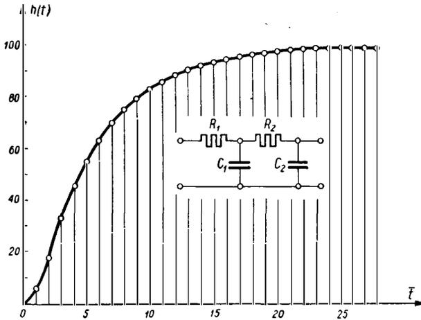
Fig. 18. Time characteristic of an RC two-section four-pole
