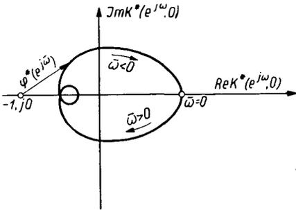
Fig. 19. Nyquist diagram of an open sampled-data control system
