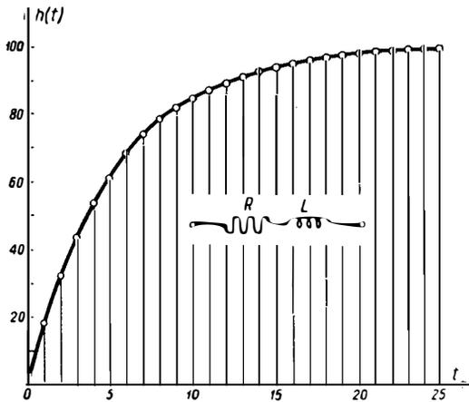
Fig. 16. Time characteristic of an RL two-pole
