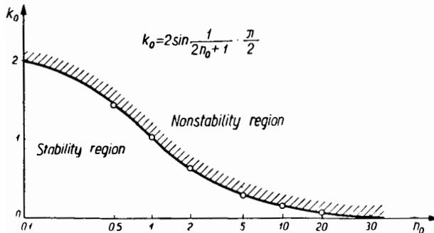
Fig. 11. Stability limit of an astatic sampled-data system
