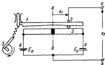
Fig. 4. Operation principle of a mechanical sampler of the first type. (1) bar, (2) indicating needle of the galvanometer, (3) winding of the resistor, (4) batteries of voltage  $E$ , (5) driving mechanism
