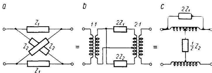
Fig. 4. Systems equivalent to a lattice four-pole
