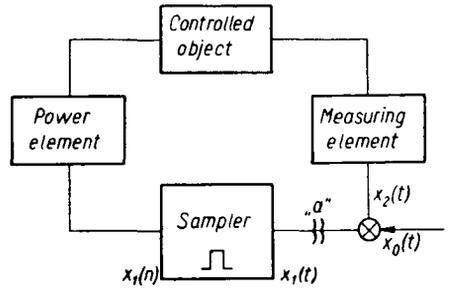
Fig. 7. Basic diagram of a sampled-data systems
