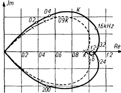
Fig. 7. The function  $K = \sqrt{\frac{Z_\alpha}{Z_\beta}}$  and  $0.9 K$
